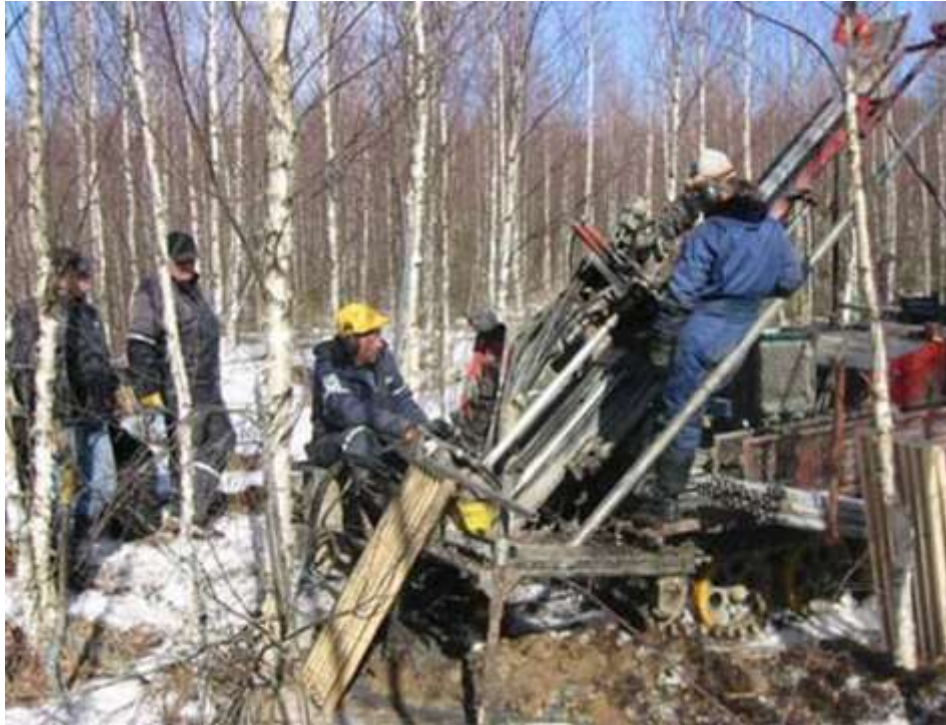
Figure 14 – Diamond Drilling on a Prospective Mine Site
